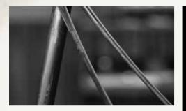
As suggested by "dual," these seat stays are a composite of two lightweight and ultra stiff materials: a composite glass fiber and carbon. The solid core provides incredible rigidity, and the carbon outer layer acts as added vibration damping. In the end, you have a bike that gives the rider a lot more control and a lot less fatigue on the ride.
