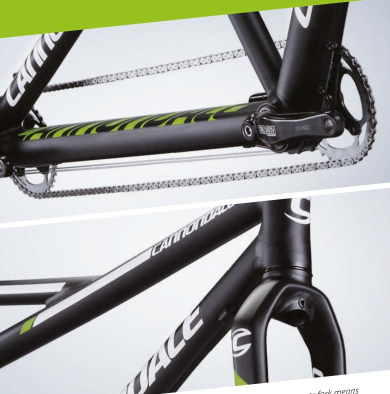
Smooth-rolling 29" wheels, trail-oriented geometry and a burly 1.5"-steerer fork means that this tandem can handle anything that comes its way, from alpine singletrack to potholed tarmac.
