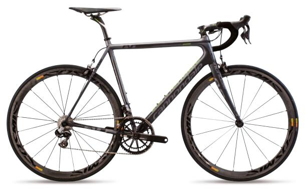
FRAMESET: SuperSix EVO, BallisTec HI-MOD Carbon, Di2 Specific WHEELSET: Mavic Cosmic Carbone 40 WTS CRANKSET: HollowGram SiSL2 w/SpideRing
