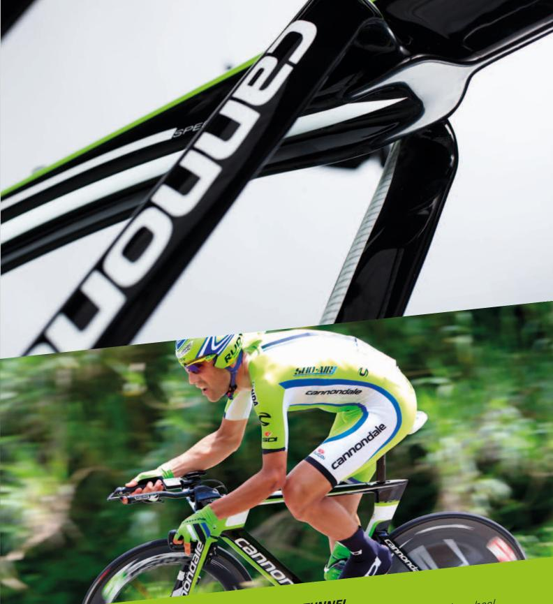
**WINDTUNNEL PRESSURE-DRAG REDUCTION TUNNEL** The WindTunnel channel behind the seat tube reduces the pressure drag on the wheel, allowing it to spin more freely.
