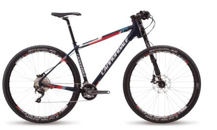
FRAME: F29, SmartFormed Alloy FORK: Lefty PBR 90 29 (90mm) RD/FD/SHIFT: Shimano SLX/Deore/SLX WHEELSET: Stan's ZTR Rapid 29 / Shimano M525 BRAKES: Shimano Deore COLOR: Mariner Blue, w/Red, White, Blue - Gloss
