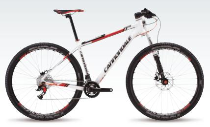
FRAME: F29, SmartFormed Alloy FORK: Lefty PBR 90 29 (90mm) RD/FD/SHIFT: SRAM X9/X7/X7 WHEELSET: Stan's ZTR Rapid 29 / X9 BRAKES: Magura MT2 COLOR: Magnesium White, w/ Red, Black - Gloss
