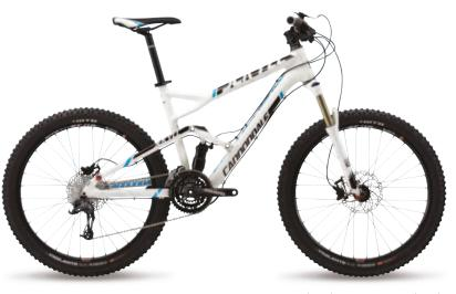
FRAME: Jekyll, SmartFormed Alloy SUSPENSION R/F: Xfusion P1-RL (150mm) / RockShox Sektor TK DPC (150mm) RD/FD/SHIFT: SRAM X7/X7/X5 WHEELSET: WTB ST 119 TCS / Formula BRAKES: Magura MT2 COLOR: Magnesium White w/ Black, Blue - Gloss
