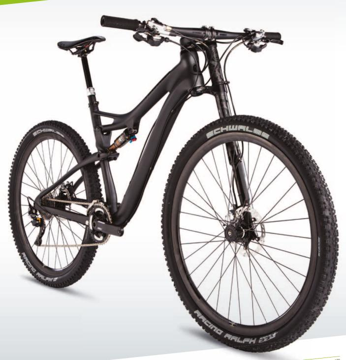
FRAME: Scalpel 29, BallisTec Hi-MOD Carbon SUSPENSION R/F: Fox Float CTD Kashima (100mm) / Lefty Carbon XLR 100 29 (100mm) RD/FD/SHIFT: Shimano XTR/SRAM XO/Shimano XTR
