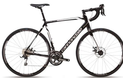
FRAMESET: Synapse Disc - Optimized 6061 Alloy, carbon bladed fork WHEELSET: Maddux RD 3.0 Disc CRANKSET: FSA Gossamer, BB30, 50/39/30 COCKPIT: Cannondale C3 CROUP: Shimano 105 / Promax Render Brakes COLOR: Jet Black w/ White - Gloss
