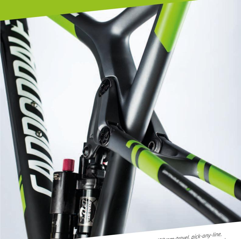
With a flick of the switch, the Trigger 29 transforms from a 130mm-travel, pick-any-line, oll-over-anything trail eater, to an 80mm-travel climbing machine. Add in the switchbackslicing SuperMax with custom offset, and you get a bike so good, it's crazy...
