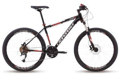
FRAME: Trail 29, double-butted 6061 Alloy FORK: SR Suntour XCM, remote lockout (100mm) RD/FD/SHIFT: Shimano Acera/Altus/Altus WHEELSET: Alex DC 4.0 / C4 BRAKES: Cannondale Helix 6B hydraulic COLOR: Jet Black, w/ White, Red - Gloss
