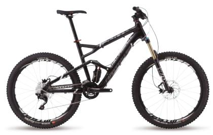
FRAME: Jekyll, SmartFormed Alloy SUSPENSION R/F: Fox DYAD RT2 (150/90mm) / Fox 34 Float CTD 0/C (150mm) RD/FD/SHIFT: Shimano XT/SRAM X7/Shimano SLX
