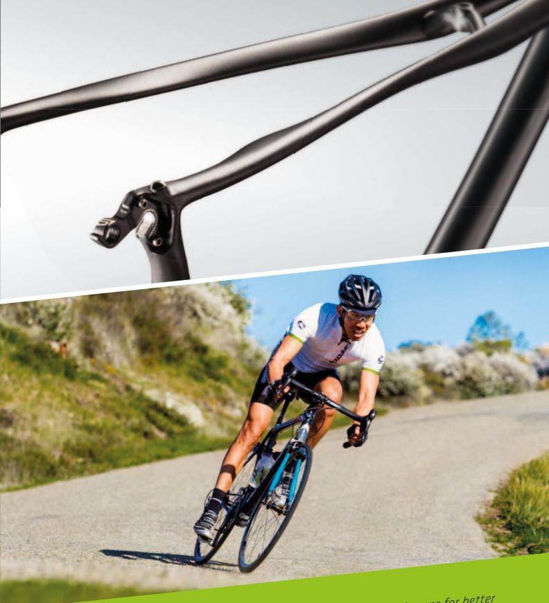
**SAVE PLUS - REAR TRIANGLE** The helixed shapes of the rear stays work with the fork to absorb bumps for better comfort and control. The seat tube and 25.4mm seatpost flex together for additional comfort in the saddle.
